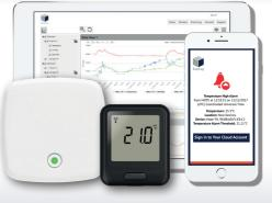
Lascar's range of temperature & humidity EL-WiFi devices connect to the EasyLog Cloud and send data from your environment. They feature a large LCD display and can be battery or mains powered. The wireless EL-MOTE family provides a discreet solution without a display and has a built in sounder and LEDs providing an efficient alarm function. It's replaceable probes offer continued logging without recalibration down time.
