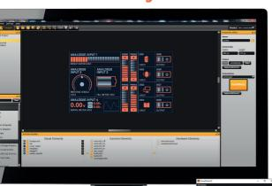
Design Studio is Lascar's free drag-and-drop software which you can download from our website. It saves you writing a single line of code, and can be used with both the 4.3" and the 7" version of the PanelPilotACF
